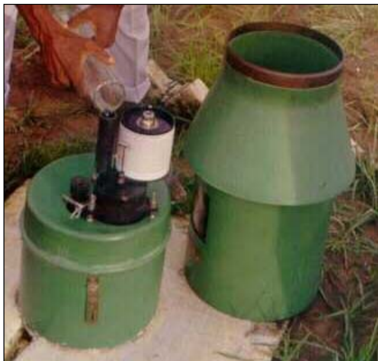
Figure 2.2: Installation of natural siphon recording rain gauge
