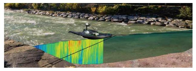
FIGURE 3.21: AN ADCP AND A TETHERED FLOAT
