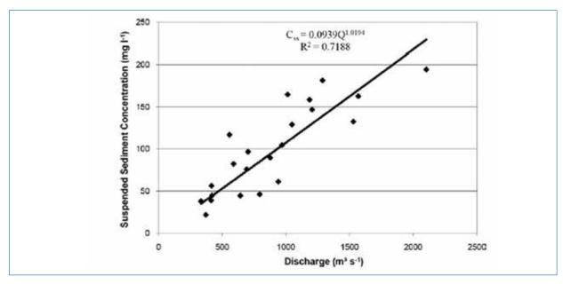
**FIGURE 6.2: A TYPICAL SEDIMENT TRANSPORT CURVE**
