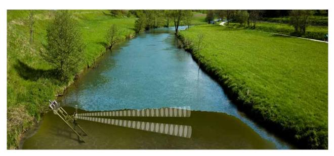
FIGURE 3.18: APPLICATION OF A SIDE-LOOKING ADCP
