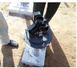
FIGURE 2.1: A) A TYPICAL TIPPING BUCKET RAIN GAUGE (TOP); B) A 0.5 MM BUCKET INSTALLED DURING HYDROLOGY PROJECT (HP)-II (ABOVE)
