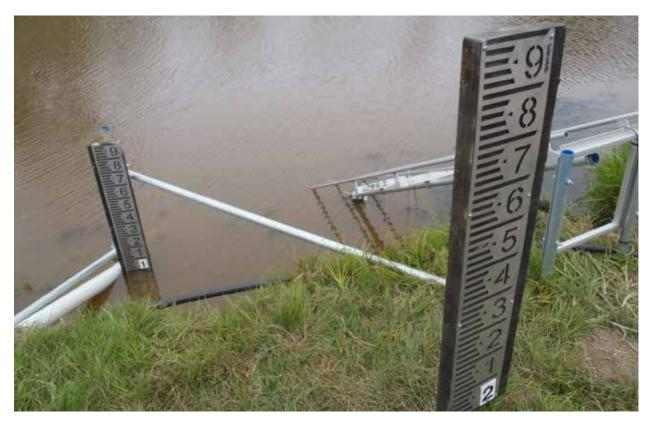
FIGURE 3.2: A STAFF GAUGE IN TWO SECTIONS
