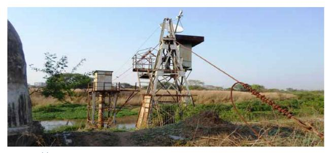
FIGURE 3.23 (B): A MANUALLY OPERATED CABLEWAY INSTALLED IN MAHARASHTRA
