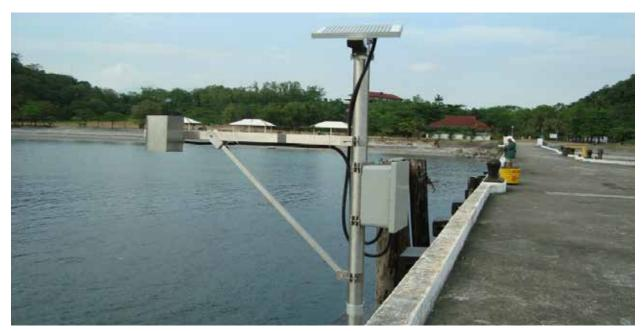
FIGURE 3.5: AN ULTRASONIC SENSOR WITH A BOOM MOUNT
