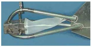
FIGURE 6.4: HALLEY SMITH BEDLOAD SAMPLER
