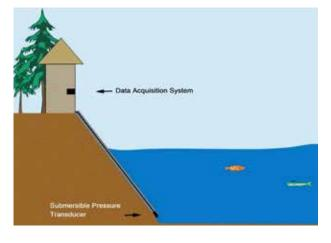
FIGURE 3.13: A SUBMERSIBLE PRESSURE TRANSDUCER INSTALLATION
