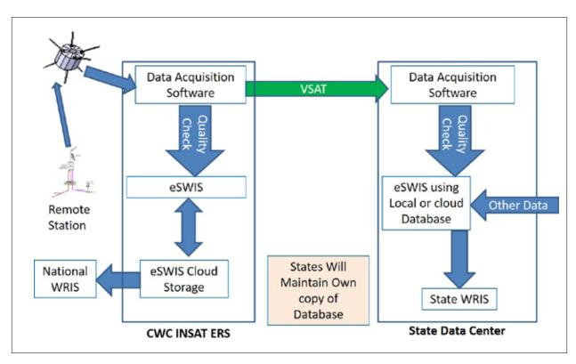
FIGURE 8.4: DATA FLOW FOR INSAT COMMUNICATION USING CWC ERS
