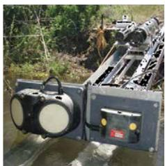
FIGURE 6.6: AN ILLUSTRATION SHOWING THE USE OF AN ACOUSTIC DOPPLER VELOCITY METER IN CONJUNCTION WITH A SUSPENDED SEDIMENT SAMPLER FOR CONTINUOUS MONITORING OF SUSPENDED-SEDIMENT CONCENTRATION
