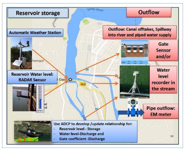
FIGURE 10.1: A TYPICAL LAYOUT FOR INTEGRATED RESERVOIR MONITORING
