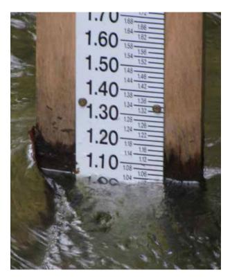
FIGURE 3.1: ESTABLISHMENT OF DATUM USING A STAFF GAUGE
