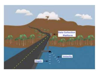
FIGURE 3.19: DOWN-LOOKING DOPPLER RADAR MEASUREMENT OF SURFACE VELOCITY COMBINED WITH ULTRASONIC DEPTH OF WATER
