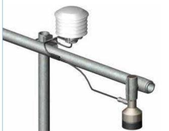
FIGURE 2.5: A) A SNOW DEPTH SENSOR SHOWING THE TEMPERATURE COMPENSATION DEVICE (LEFT); B) AN INSTALLATION WITH AN INDEPENDENT TEMPERATURE SENSOR (RIGHT)
