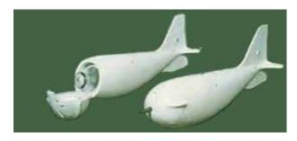
FIGURE 6.3: A DEPTH-INTEGRATING SUSPENDED SEDIMENT SAMPLER
