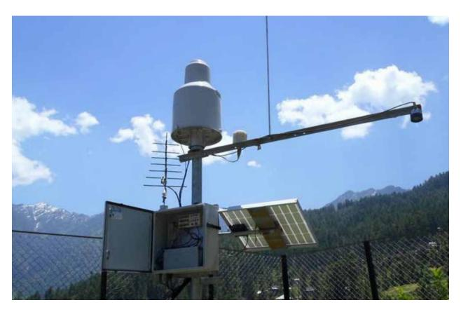
FIGURE 2.4: A PRECIPITATION GAUGE INSTALLED IN MADANA, HIMACHAL PRADESH, BY THE BHAKRA BEAS MANAGEMENT BOARD
