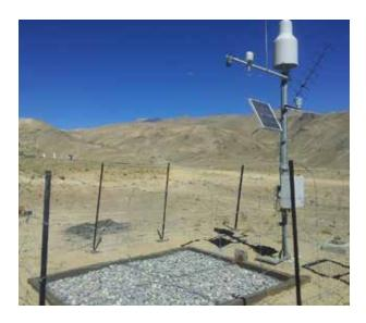
FIGURE 2.6: B) A SNOW MEASUREMENT STATION.
