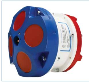
FIGURE 3.20: AN ACOUSTIC DOPPLER CURRENT PROFILER
