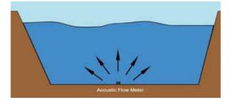
FIGURE 3.17: THE SCHEMATIC OF AN UPWARD-LOOKING ADCP
