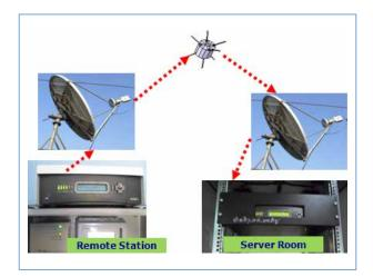
FIGURE 8.5: SATELLITE-BASED COMMUNICATION USING VSAT
