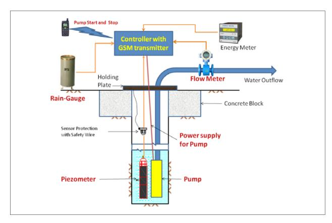
FIGURE 9.1: INTEGRATED GROUNDWATER MONITORING
