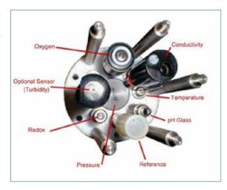
FIGURE 5.1: MULTI-PARAMETER WATER-QUALITY SONDE WITH SENSORS
