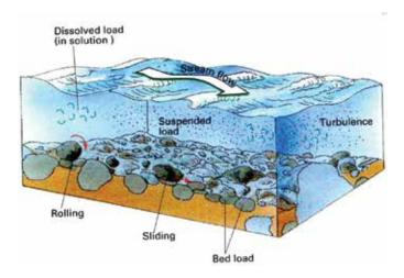
FIGURE 6.1: AN ILLUSTRATION SHOWING THE VARIOUS MODES OF SEDIMENT TRANSPORT IN A RIVERINE SYSTEM
