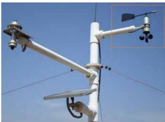
FIGURE 2.9: AN ULTRASONIC WIND VELOCITY AND DIRECTION SENSOR (LEFT) AND A CUP-ANEMOMETER AND WIND VANE-BASED WIND VELOCITY AND DIRECTION SENSOR (RIGHT)
