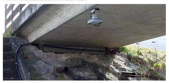
FIGURE 3.6: AN ULTRASONIC SENSOR BEING USED TO MEASURE WATER ELEVATION USING A BRIDGE MOUNT
