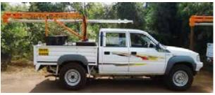
FIGURE 3.26: A VEHICLE-MOUNTED CRANE FOR DEPLOYMENT OF ADCP FROM A BRIDGE
