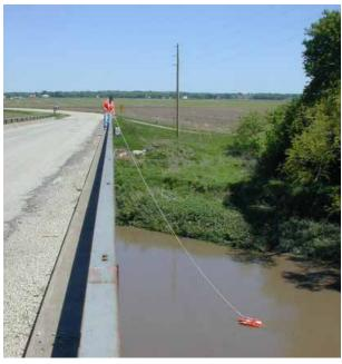
FIGURE 3.25: DEPLOYMENT OF AN ADCP FROM A BRIDGE
