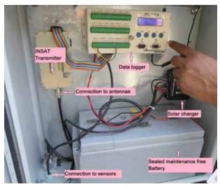
FIGURE 7.2: EQUIPMENT INSTALLED INSIDE THE BOX ON THE DCP
