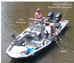
FIGURE 3.24: DIFFERENT ADCP DEPLOYMENT OPTIONS USING BOATS
