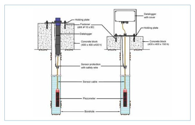
FIGURE 4.1: C) AUTOMATIC WATER-LEVEL SENSORS WITH AN INTERNAL DATA LOGGER AND EXTERNAL DATA LOGGER FOR MULTI-PARAMETER MONITORING AND TELEMETRY
