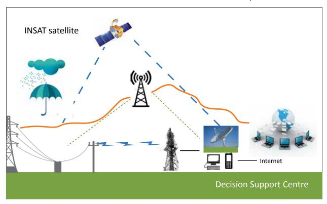
FIGURE 8.1: EXAMPLES OF VARIOUS TELEMETRY SOLUTIONS FOR THE RELAY OF REAL-TIME HYDROLOGIC INFORMATION
