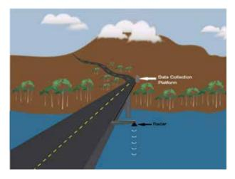
FIGURE 3.7: A RADAR SENSOR WITH A BRIDGE MOUNT
